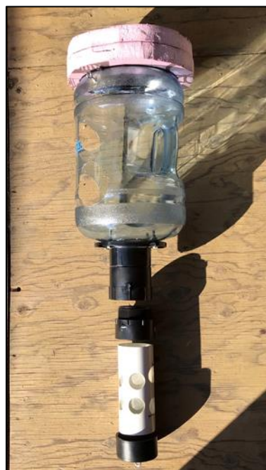
Figure 5. Main body of trap with foam float attached and cod end pieces staged for assembly.
