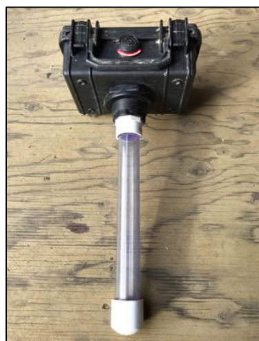
Figure 7. Light housing consisting of Pelican box, bulkhead fitting, and capped PVC pipe.
