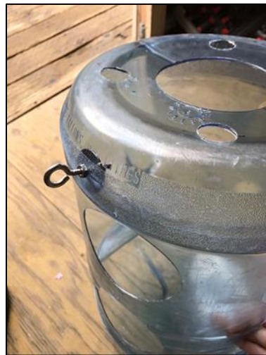
Figure 4. Main body of trap with holes drilled in the side and bottom. Stainless steel eye bolts are used to strap the foam lid and handle to the trap.
